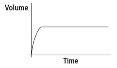
Following a normal start to the procedure the trace reaches an abrupt plateau. Actual FVC is not reached.
